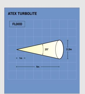
A-TL44A/B - Ball Glass Peak luminous intensity at 2.5m 70lux
