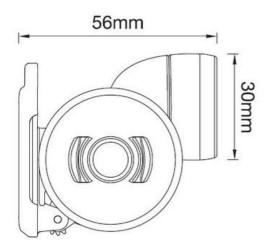
High Power LED spot beam (approx 22°) Peak luminous intensity at 1m **493 lux**, at 2.5m **67 lux** Extra wide angle fringe beam (approx 100°) Peak luminous intensity at 1m **32 lux**, at 2.5m **8 lux**
