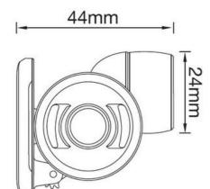
High Power LED spot beam (approx 20°) Peak luminous intensity at 1m 381 lux, at 2.5m 52 lux Extra wide angle fringe beam (approx 85°) Peak luminous intensity at 1m 25 lux, at 2.5m 6 lux
