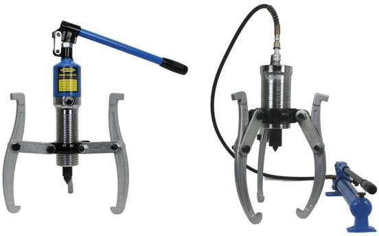
Hydraulic bearing pullers are used to easily remove bearings in different situations. These can be supplied with a separate or with a build in hydraulic pump. Available in different sizes and outputs. Can be used as 2 and 3 arm configuration.
