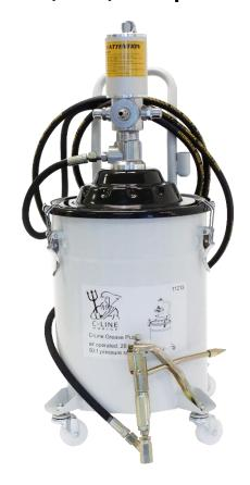
Accessories: 4 meter grease hose, grease gun with triple swivel, spare part set
